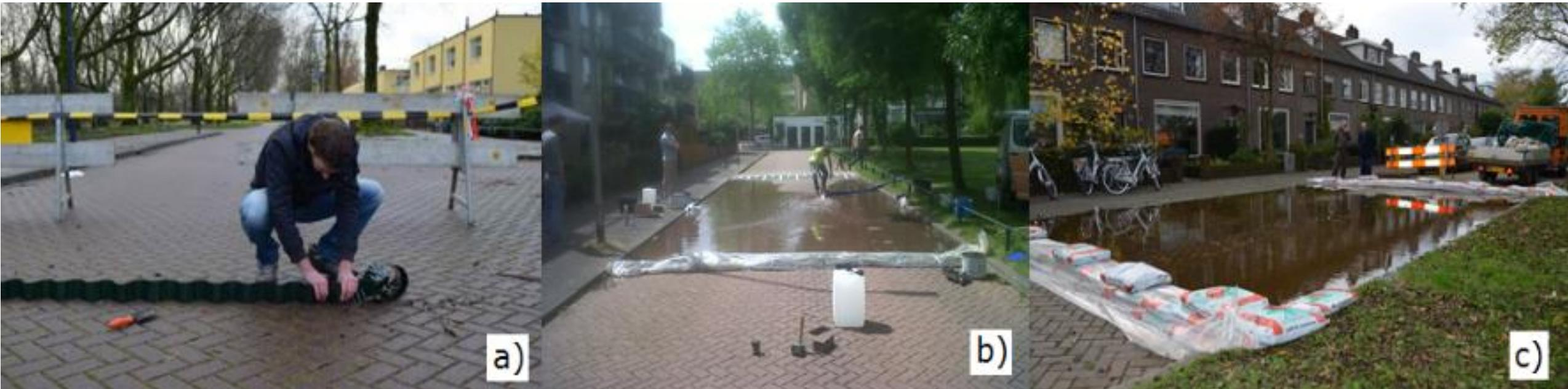
Various Dam Variations Used at the Different Test Locations (a) Impermeable barriers; (b) Plastic wrapped soil core; (c) Soil-filled plastic bags. [share](#) your talent. [move](#) the world.
