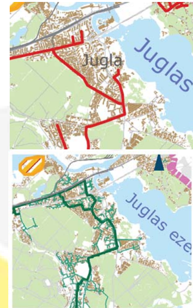
Pic.7, Gas supply grid (above) and district-heat supply grid (below) in Jugla
